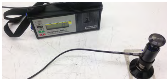
Figure 12. Adhesion Test Using ASTM D4541
