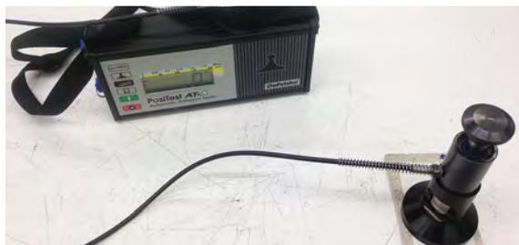
Figure 12. Adhesion Test Using ASTM D4541
