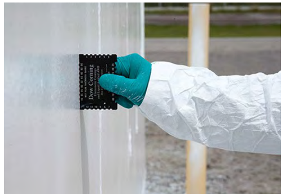
Demonstrating usage of wet mil gauge
