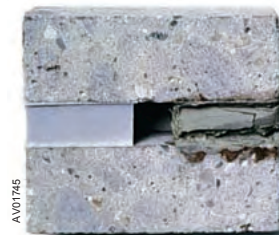
After 100 days (2,400 hours) of UV exposure in accelerated weathering and heat stability tests, the urethane sealant deteriorates, while the silicone sealant remains untouched.
