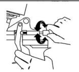
Adjust bead with gun regulator screw.
