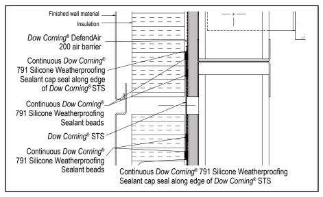
Figure 12. Deflection joint at intermediate floor slab; wall passes in front of slab.
