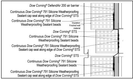
Figure 13. Deflection joint at intermediate floor slab; slab interrupts wall.
