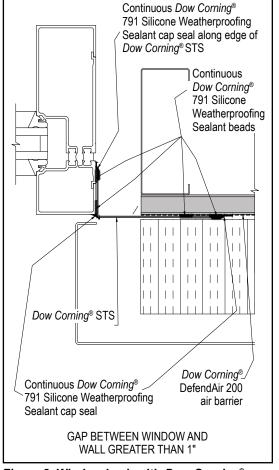
Figure 8. Window jamb with *Dow Corning*<sup>®</sup> Silicone Transition System detail.
