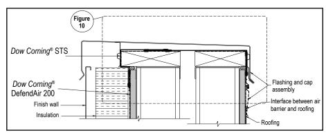
Figure 14. Parapet wall cap detail.
