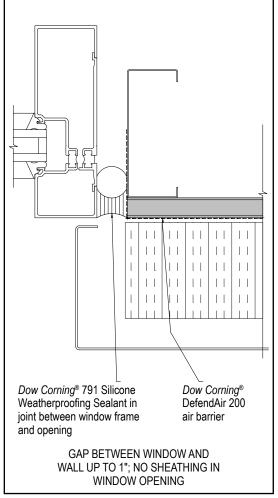
Figure 7. Window jamb with sealant detail.
