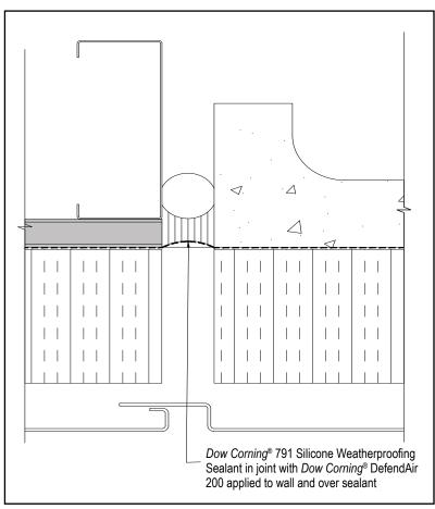
Figure 3. Change in substrate detail.
