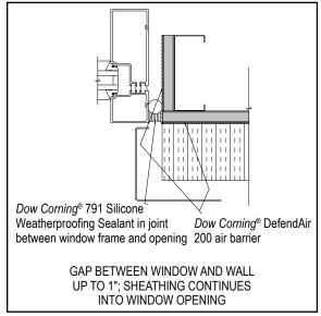
Figure 15. Window jamb condition.
