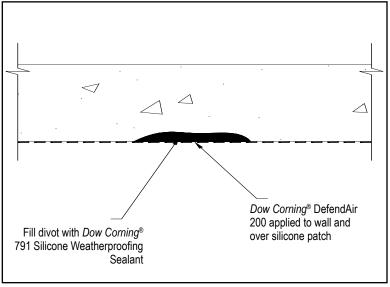
Figure 2. Divot in concrete wall detail.
