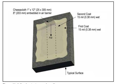
Figure 11. Adhesion test procedure diagram.
