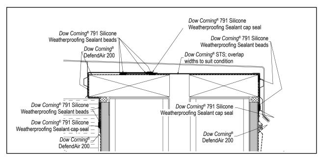
Figure 10. Dow Corning® Silicone Transition System under cap.
