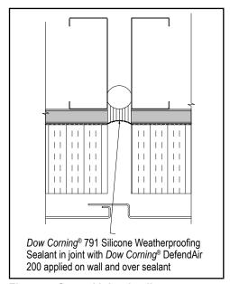
Figure 4. Control joint detail.
