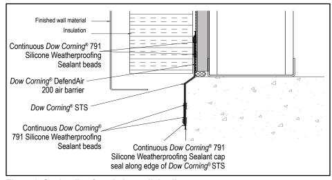
Figure 9. Stud wall to foundation wall detail.
